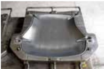
Molds for the <5_MY seat await layers of hand-assembled carbon fiber sheets that will become the light—but incredibly strong—chair frame.
